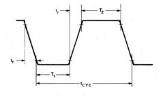
Figure 2. Clock Specification for 8755A
